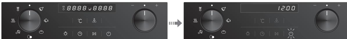
**Note:** If no operation after a few minutes, it switches to the off state. All indicators light out (except the “☀️, ⏻” buttons, press any other button, “⏻” button flashes).
