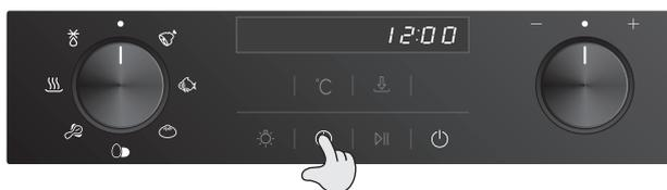
**Note:** The default time is 12. If the power is disconnected for a few seconds, the time will return back automatically to the default time 12:00 again. Time needs to be reset after the appliance is plugged in.
