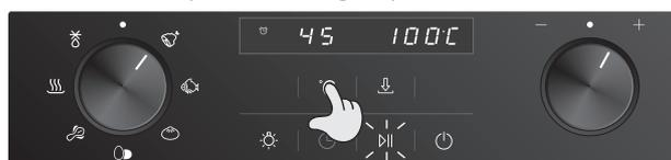
Set the cooking time. Press the “⌚” button and the time display section flashes, Then rotate the “right knob” to set the time needed (see below figure).
