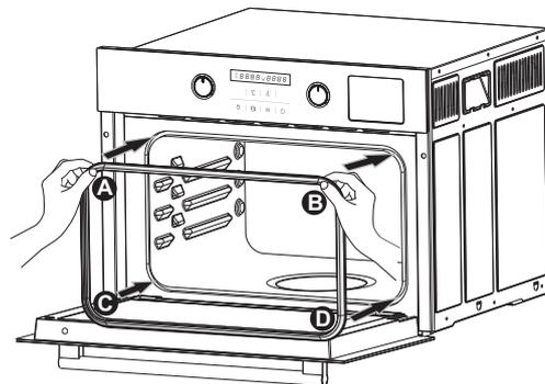
Hold the A & B half circle at the upper area of the door seal by hands. Align to the half circle slots at the upper area of the front panel and press in tightly. Then align the C & D half circles at the bottom to the two slots at the bottom of the front panel and press in tightly. Press the four sides completely into the slots. Make sure the seal is flat, not wrinkled and no gap.
