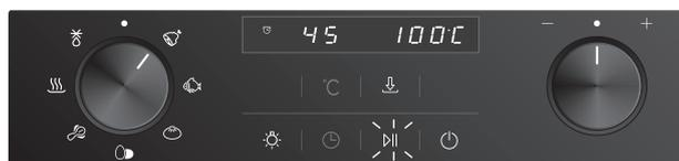
Set the cooking temperature. Press “°C” button and the temperature display section flashes, Then rotate the “right knob” to set the temperature needed (see below figure).
