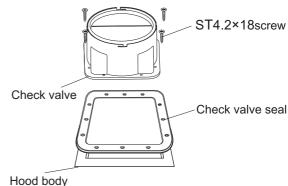
●Installation of check valve: As shown in the figure, fix the check valve sealing ring and check valve at the air outlet at the top of the body with 8 ST4.2 × 18 self-tapping screws.
