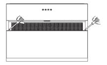
Turn the 2 screws on the left and right sides of the protective net counterclockwise for 3-5 turns with a Phillips screwdriver.
