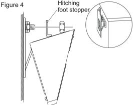
●Installing the machine body: Install the machine body into the hanging leg (the hanging hole is on the upper side of the back of the machine body). after the machine body is aligned, install the hanging leg limiting block and tighten the nut (to prevent the machine body from unhooking under the action of external force).
