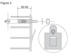
●Installation of hanging feet: Drill holes at a certain position with a hole depth of 50-55mm and a hole diameter of 10mm (not too large). Insert M6 metal expansion pipe into the hole, install hanging feet, gaskets and tighten nuts.
