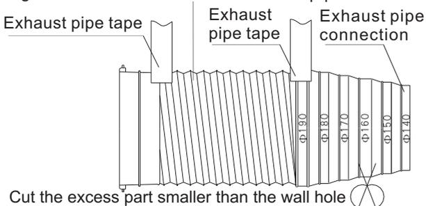
**Note: During installation, straighten the aluminum foil exhaust pipe to avoid noises in semi-stretched state. Excess part may be cut with a wire cutter.**
