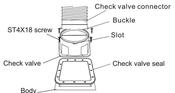
The exhaust wall hole diameter shall be close to that of the exhaust pipe, which shall not be too small. Otherwise, it will cause poor exhaust efficiency, more noises and lower airflow, etc. The connection between the pipe and the hole or the public flue must be sealed tightly to ensure that, the pipe and the check valve or public flue are connected securely. The blades at the check valve connection or public flue connection must be flexible.
