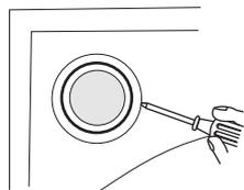
Insert a small flat head screwdriver or something sharp in the gap between the light cover and hood.
