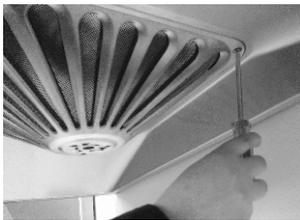
Align the cross screwdriver with the screw hole and raise it upward forcibly meanwhile rotating it counter-clockwise about 120°, so as to remove the screw out of the cross slot of the exhaust fume collecting hood. Hold the bottom of the mesh with one hand, and remove the screw on the other side with the other hand by the cross screwdriver.
