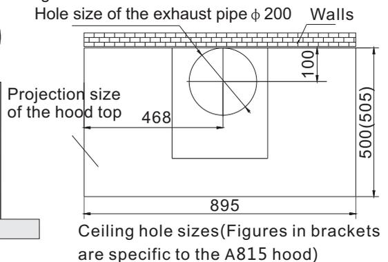
Ceiling hole sizes (Figures in brackets are specific to the A815 hood)
