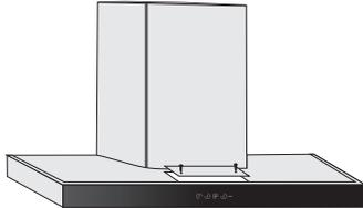
Untighten two screws on the small plate to remove the plate.
