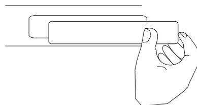
Raise the spotlight outward forcibly to remove it from the hood. Pull out the connector to replace the spotlight.
