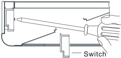
After removing the spotlight, remove the two screws on the switch with a cross screwdriver and move the switch assembly diagonally upward to take it out from the lamp hole for repair and replacement.
