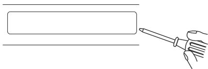
Insert a small flat head screwdriver or something sharp in the gap between the light cover and hood.
