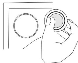
Raise the spotlight outward forcibly to remove it from the hood. Pull out the connector to replace the spotlight.
