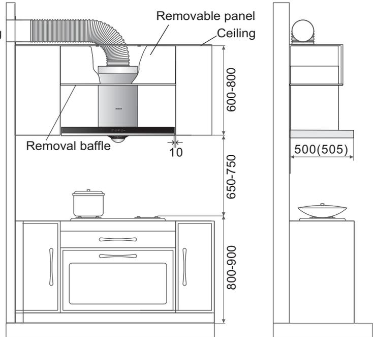
(Figure 1-2 Installation method of hood with removable baffle)
