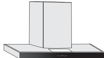
Remove the two screws on the switch cover plate and then rotate the cover plate to pull out the switch assembly for maintenance and replacement.
