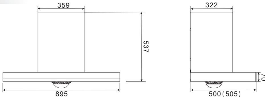
The marked sizes are for reference only. The height of drawing panel is 430, and the size in brackets is specific to A815 hood. (Unit: mm)
